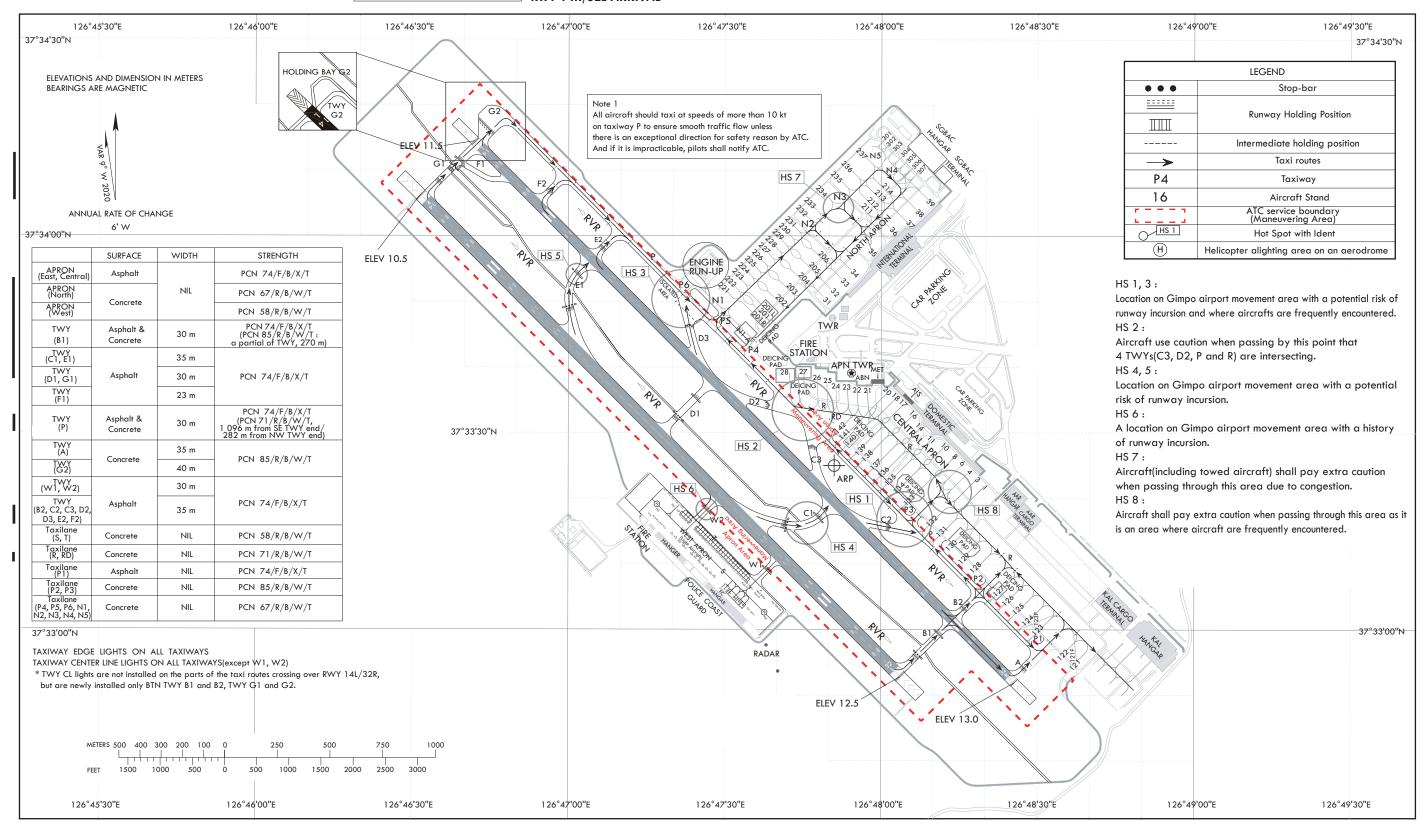
$Change: Establishment of taxilane \ RD \ and \ Information of \ TWY, lead \ in \cdot lead \ out \ line, intermediate \ holding \ position.$
